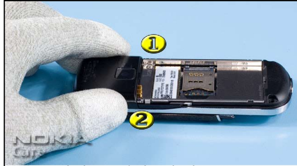
10. Unscrew both screws in the order shown.
